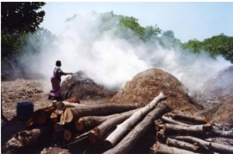
Figure 1. Traditional charcoal making uses dirt covered mounds to exclude air.
